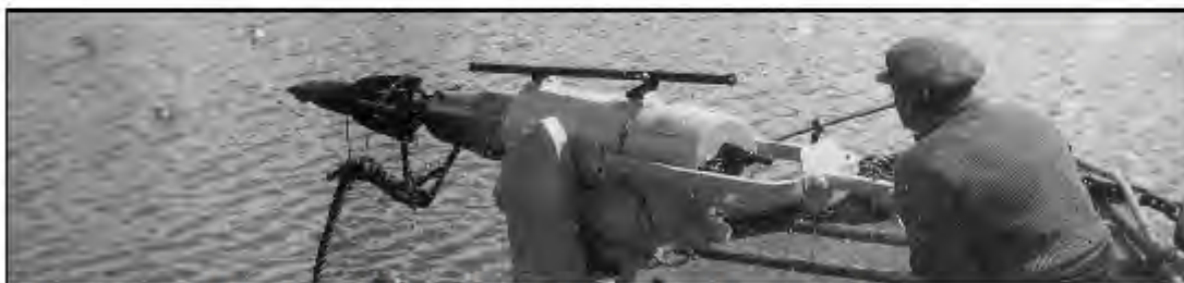
A harpoon cannon ready to fire. The gunner or 'skytter' (pronounced 'sbooster') takes aim along the sighting rod.
