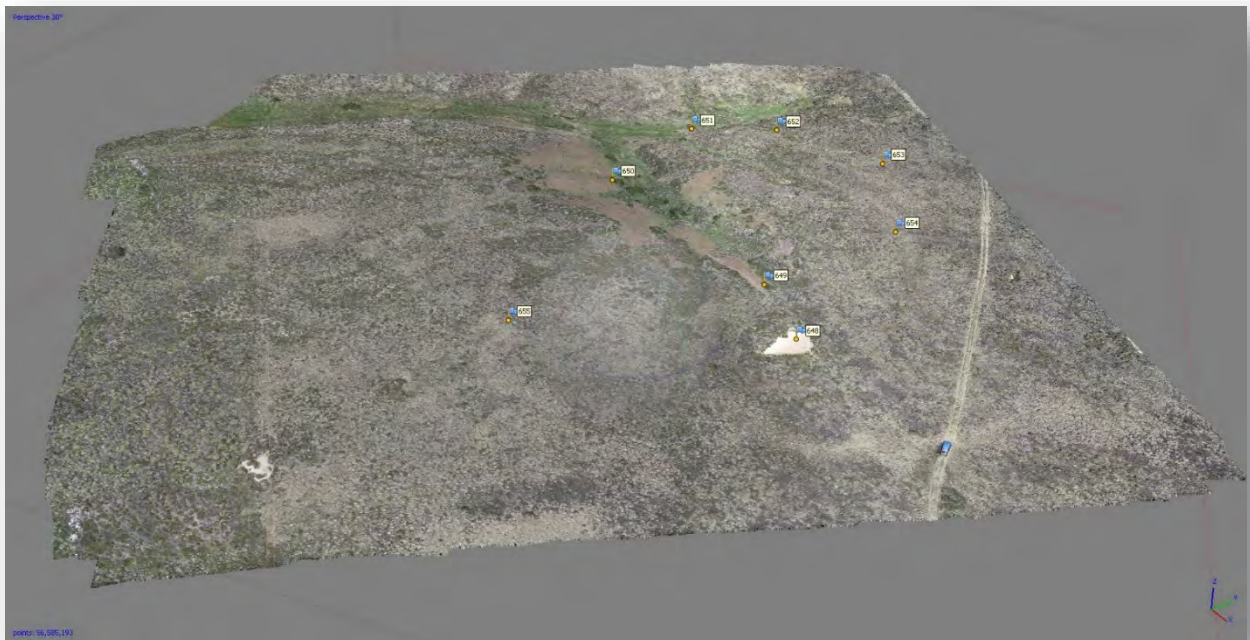
Figure 3.5.1: 3D dense point cloud (from processed drone imagery) from a calafate mapping mission at Port Sussex, East Falkland.
