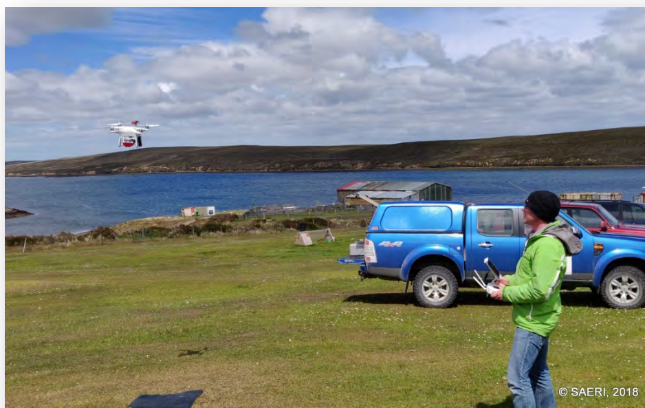
Figure 18.11: Completing drone mapping missions with a multispectral camera, focussing on calafate at Port Sussex farm.
