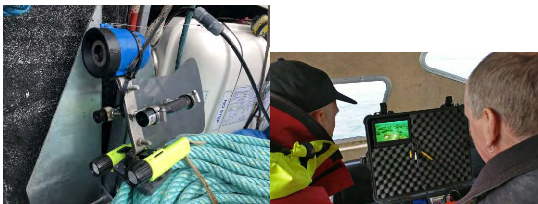
Figure 4: Example of simple drop camera (left) and live feed and recording unit (right).
