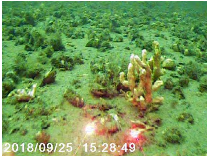
Figure 5: Live image from a drop camera. note the two laser lights to provide scale. Also note date and time imprinted on the video.
