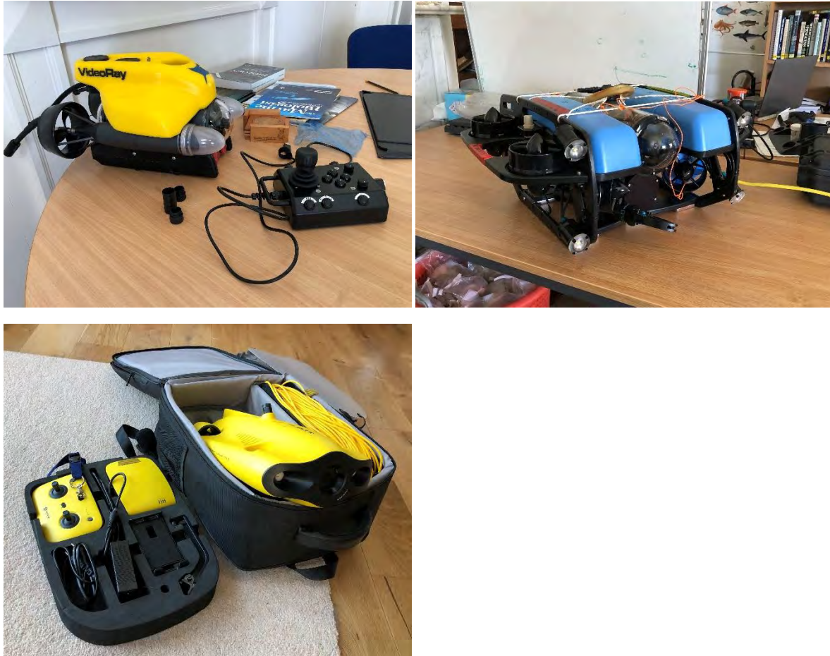
Figure 6: A range of small portable ROVs on the market; Top left – relatively expensive, off the shelf, highly capable, adaptable, low level of technical expertise. Top right – mid price, open source, highly adaptable, requires higher level technical expertise to operate. Bottom - least expensive, basic capabilities, easy to operate, low level of technical expertise, highly portable but limited by battery power.
