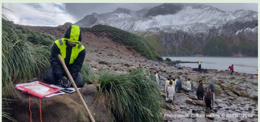
Deploying ground control points at Elsehul. These allow accurate digital elevation models to be created for specific areas, such as the area being investigated by the archaeological team of the South Georgia Archaeological Project.
