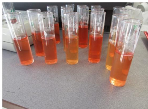
Test for magnesium; the stronger the orange, the higher the magnesium content in the soil.
