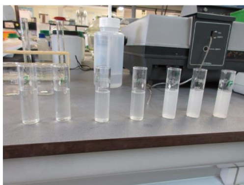
Test for potassium; the cloudier the solution, the higher the potassium content in the soil sample.
