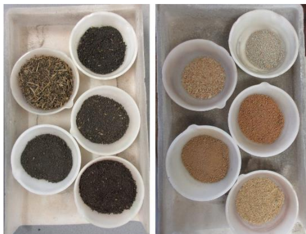
Determining the organic matter content of the samples; dried samples on the left and ash after several hours in the furnace on the right.
