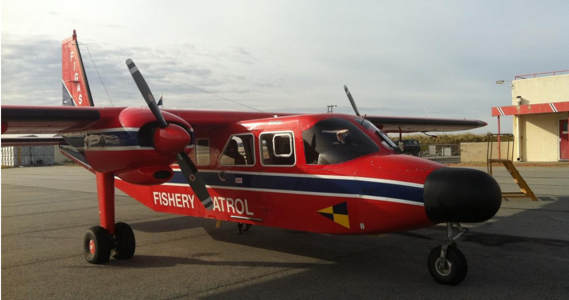
Figure 2 – The aircraft BRAVO-OSCAR used for the survey was a Britten-Norman BN-2B Islander from FIGAS.
