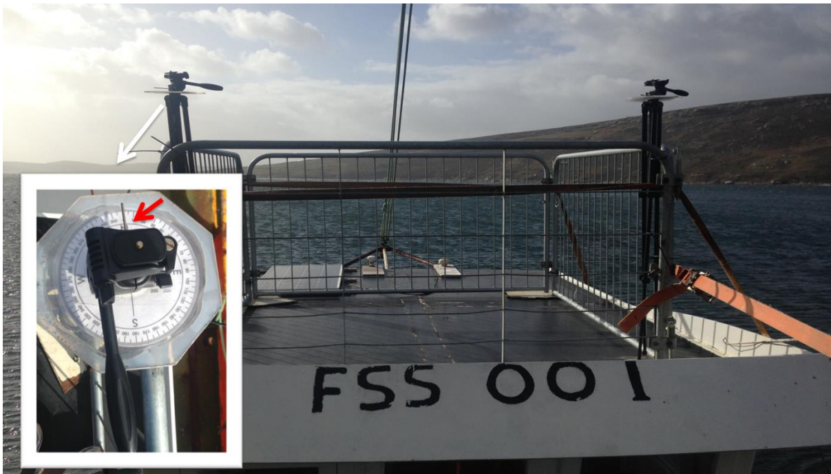
Figure 5 – Detail of the protractor. Note the protractor needle (red arrow) used to locate the bearing at which animals were sighted (bottom left enhancement box - pointed by the white arrow).
