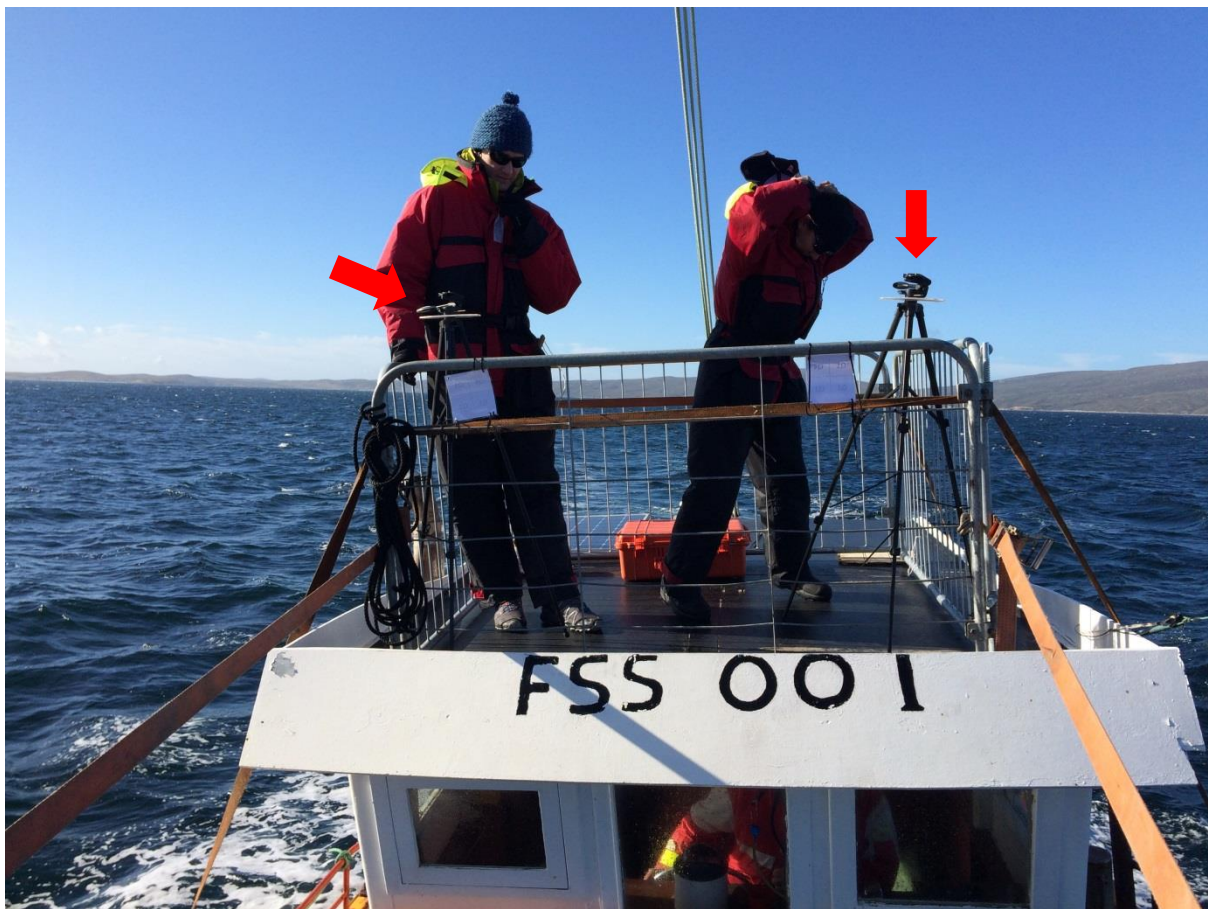
Figure 3 – Observers on the observation platform, on top of the captain cabin; a fence was set up to safely accommodate the observers. Note the presence of the protractors (red arrows) to estimate the dolphin angle at sighting.
