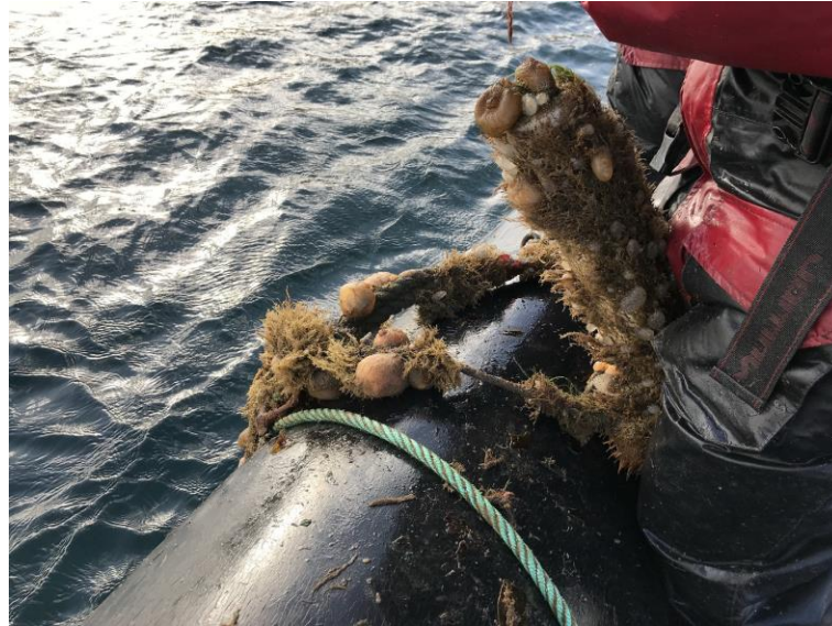
Figure 4 – Recovered C-POD unit 2020 showing thick cover of marine invertebrates (e.g. Tunicata).
